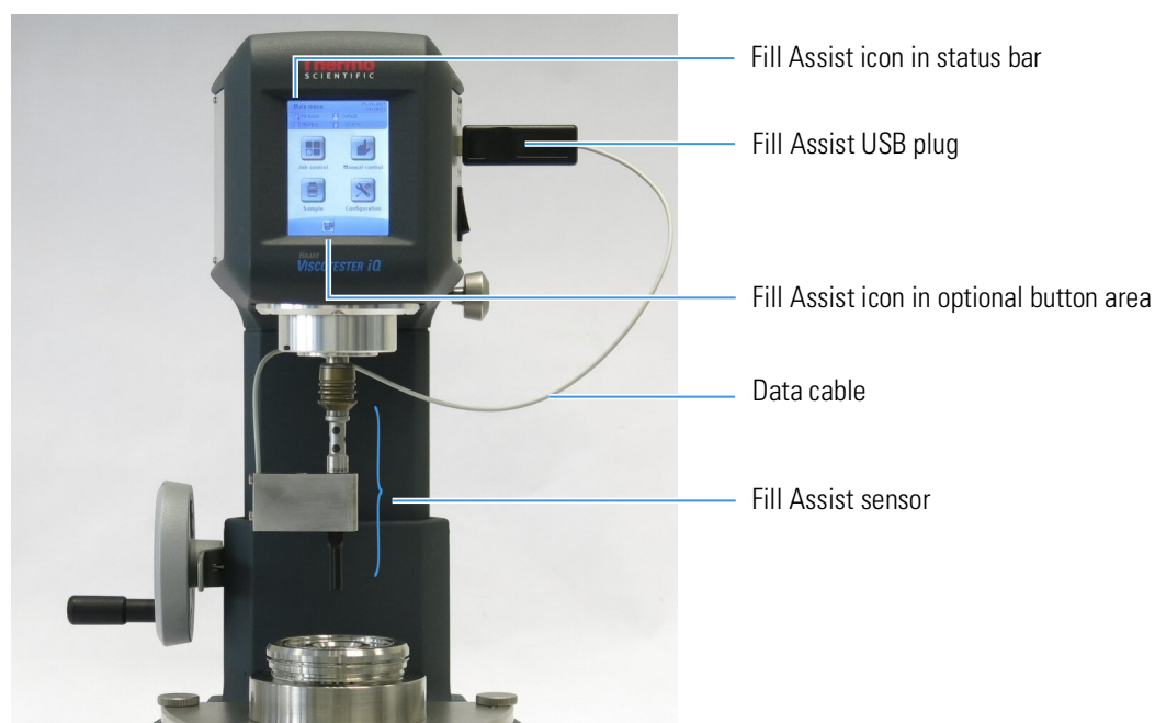
Figure 145. Fill Assist hardware mounted to the Viscotester iQ
