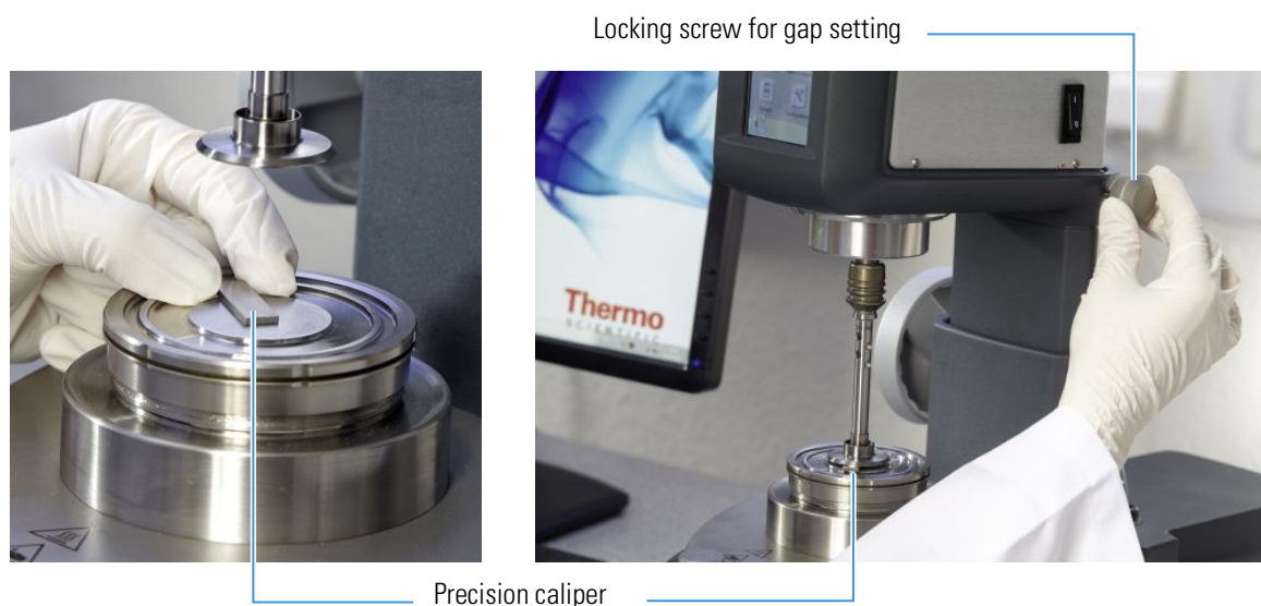
Figure 29. Using a caliper to set the gap
